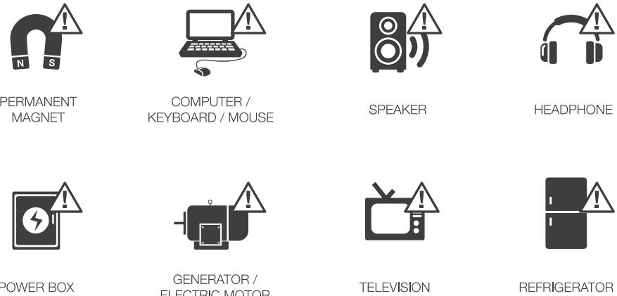
The Perception Neuron PRO system should NOT be used in an environment with strong magnetic interferences. Using the system in such an environment introduces significant errors to the motion capture results. Exposing sensors to such an environment for a long time will cause sensor magnetization.
